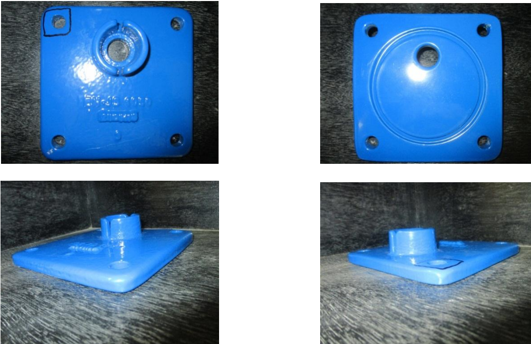
Fig 2: ISO Valve Bonnet (Before test)
