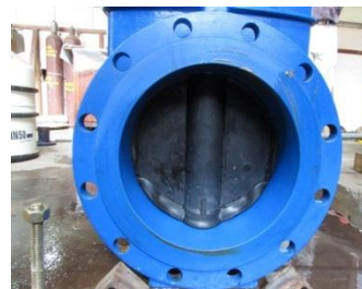
Fig 3 Low Pressure Seat Leakage Test
