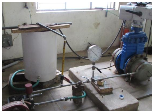
Fig 1: Test Setup (Endurance cycle testing)
