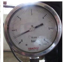
Fig 3 Low Pressure Seat Leakage Test
