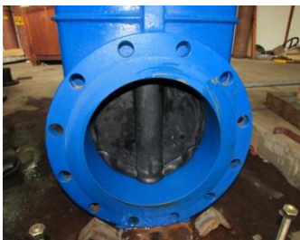
Fig 2 High Pressure Seat Leakage Test
